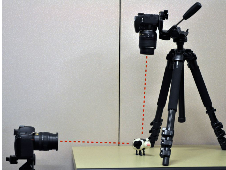
Two-camera stereo setup with the cameras at 90 degrees relative to one another.
