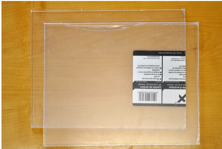
Thick plexiglass (0.22") works well as a flat surface for high-accuracy applications.
